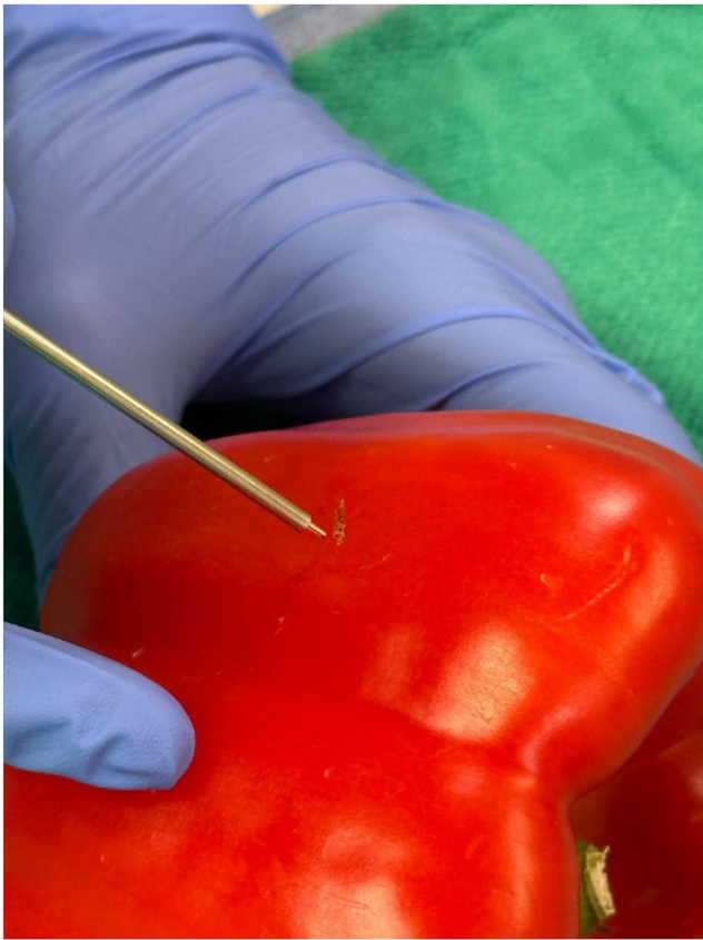
Fig. 6 Surgical Simulation with CO2 laser using a bell pepper to test various energy settings for coagulation and cut features. Courtesy of Dr. Dietrich
